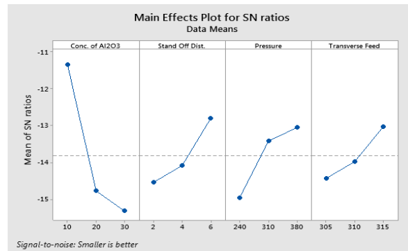
Fig. 4. Main effect plot for S/N ratios (Surface Roughness)
