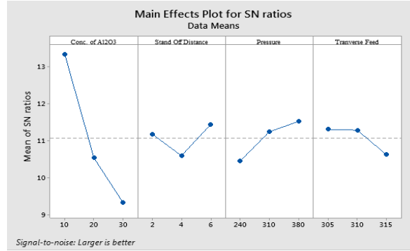
Fig. 3. Main effect plot for S/N ratios (MRR)
