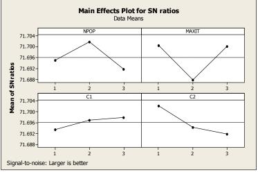
Fig. 4. S/N rate for PSO algorithm coefficients
