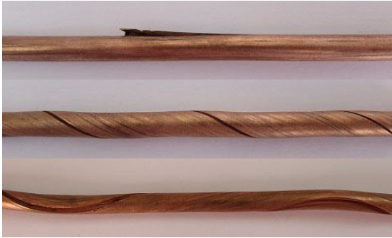
Fig. 7. Samples of a copper rod with class C quality
