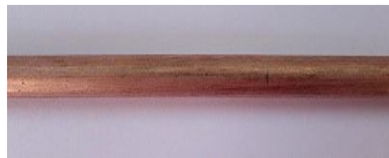
Fig. 5. Samples of a copper rod with class A quality
