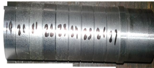
Fig. 3. Workpiece after turning the CNC machine on
