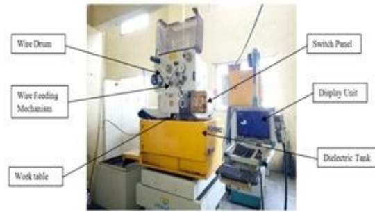
Fig. 2. Wire-Cut EDM set up photograph
