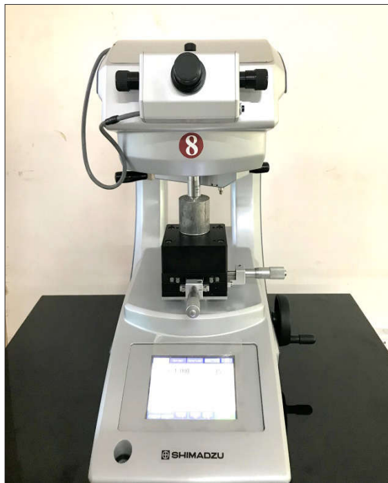
Fig. 2. Specimen loaded on (Shimadzu) hardness tester
