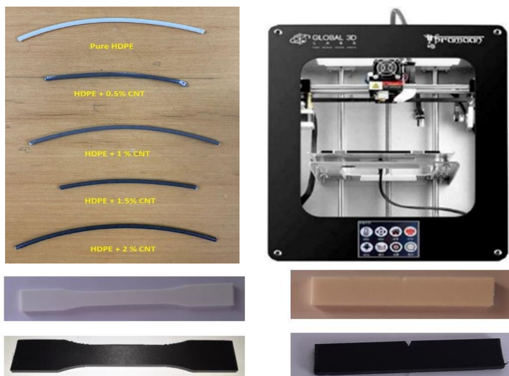
Fig. 2. (a) Photographs of filament drawn with a twin screw extruder (b). FFF printer used to print the various 3D parts (c) Tensile Test Specimen of Pure HDPE and HDPE + 2% CNT respectively (d) Impact Test Specimen of Pure HDPE and HDPE + 2% CNT.
