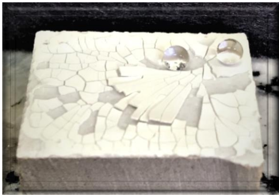
Fig. 8. Cracking and peeling of the coating, when thicker than 60 \mu\text{m} .
