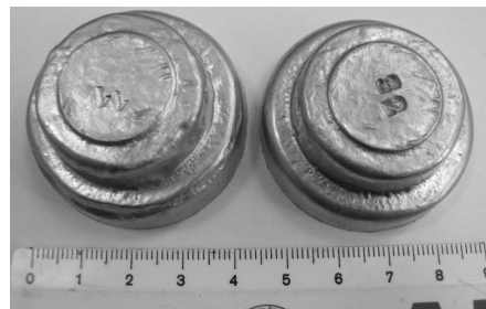
Fig. 1. Samples for testing the alloy porosity content
