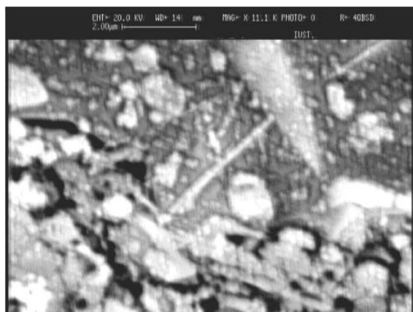
Fig. 6. Microstructure of sample without silica sol after sintering at 1400 °C showing no mullite crystals (figures 4-6), it can be concluded that the mullite
