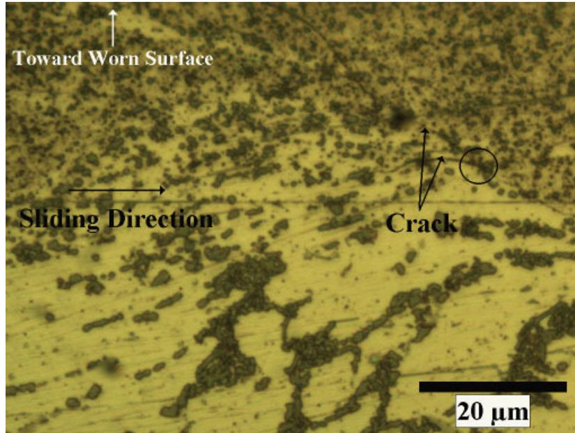
**Fig. 4.** Optical Micrograph of subsurface of worn specimen at 100N showing plastic deformation in the direction of sliding. The arrows indicate the cracks in the subsurface, and the circle suggests Al-Si eutectic led to crack deflection.
