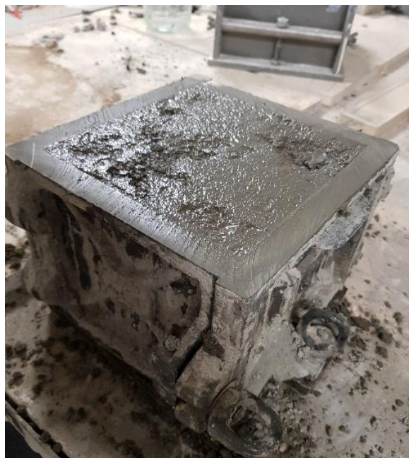
Figure 11. A 150 millimeter mold filled with concrete
